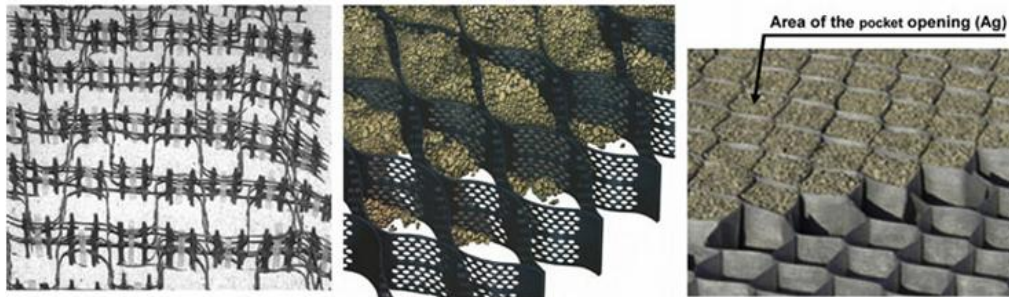
Figure 1. (a) Handmade geocells with perforations; (b) perforated geocell and (c) non-perforated flexible geocell.
