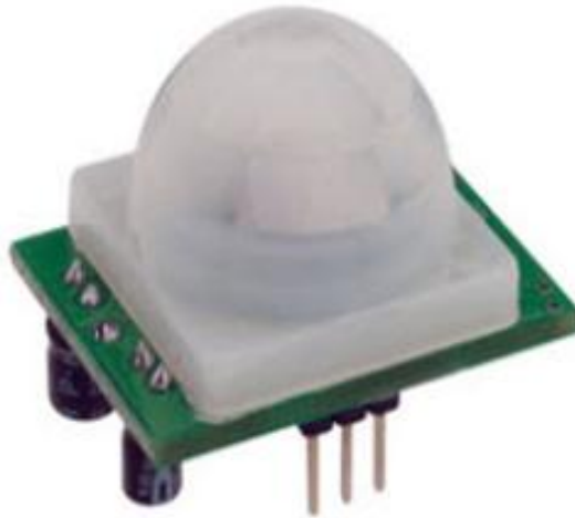
Figure 7. PIR sensor configuration with dome-shaped fresnel lens.
