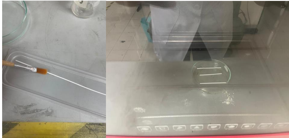
Figure 2. The process of applying alumina hollow fiber membrane with silicone and curing process using oven.
