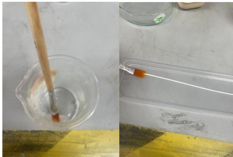
Figure 1. The process of cleaning alumina hollow fiber membrane with acetone.
